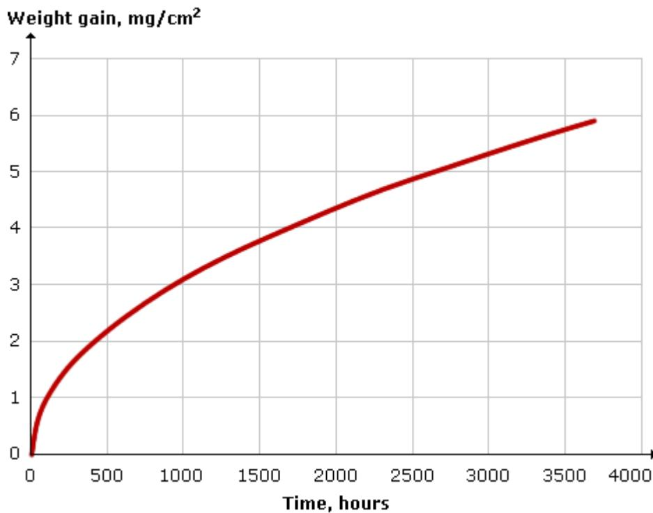
Weight gain of Kanthal APMT, due to oxide formation, when oxidized in air at 1200°C for 100h cycles with cooling to ambient temperature between each cycle.
